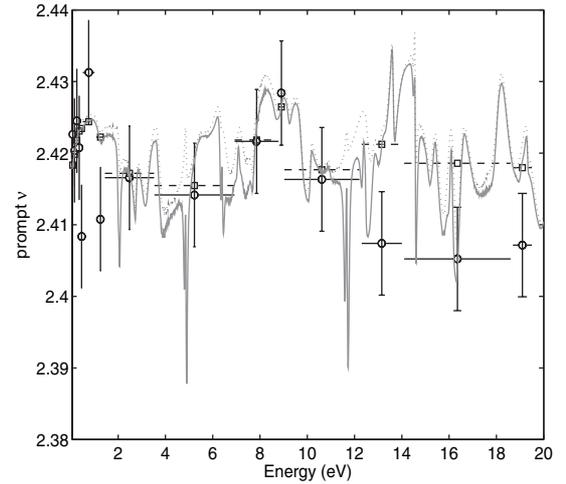
**Fig. 4.** Comparison between measured neutron multiplicity  $\langle \nu \rangle$  and calculations with the present formalism (pointwise and averaged over the same energy ranges as in the measurements). The white dots are experimental data and the white squares are the calculated values. Straight line is the pointwise calculated multiplicity and dot line is the same without (n,  $\gamma$ f) corrections.
