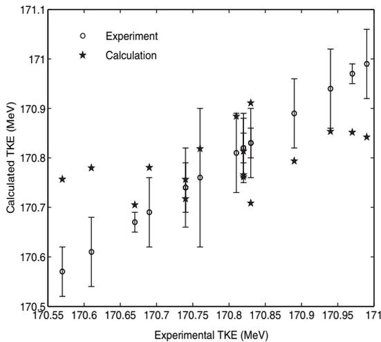
Fig. 6. Comparison between measured total kinetic energy  $\langle TKE \rangle$  and calculations with the present formalism (pointwise and averaged over the same energy ranges as in the measurements).
