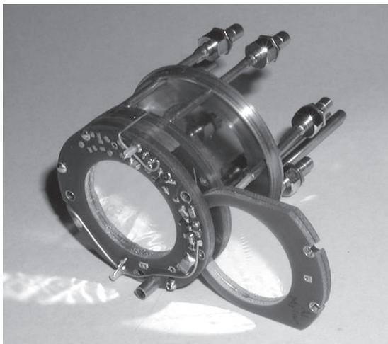
**Fig. 1.** Picture of a PPAC fission-tagging detector and the removable target/cathode foil partially inserted. The surface mount components for the first amplification stage can be seen on the front ring. The neutron beam passes through a 2.5 cm opening in the center of the G10 frame.
